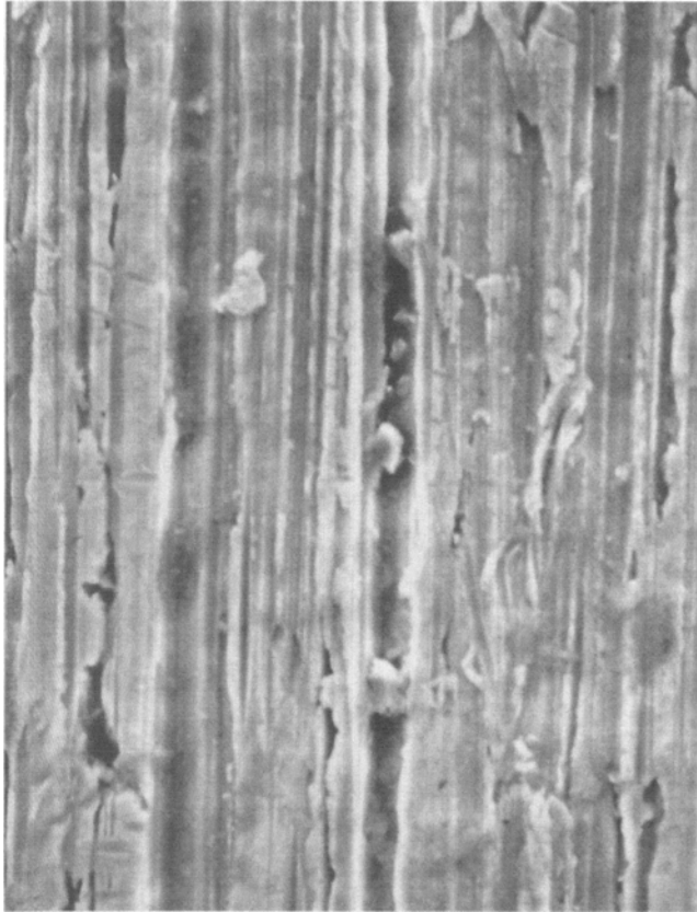
Fig. 21 SEM micrograph showing rolling marks on the surface of as-received specimen
